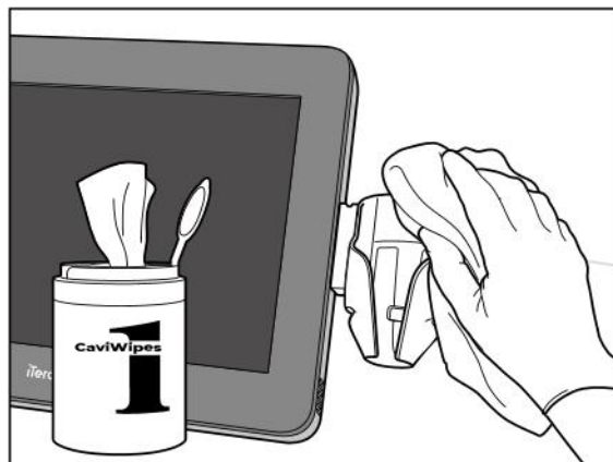
Figure 210: Wiping the iTero Element 5D Plus Lite mobile-configuration cradle
