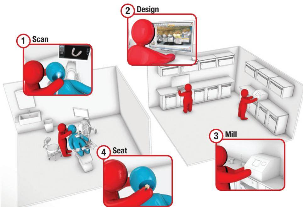
**Digital Impressions (Model Free) Workflow.** A model is no longer necessary. The accuracy of the data ensures that the designer is operating on a precise replica of the oral anatomy. Model-free digital impressions deliver an accurate, quality restoration while saving on time and lab labor.
